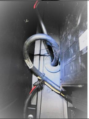
Drill a hole for the antenna cable connector / maximum diameter 9/16" based on grommet provided. If the connector is already on the antenna, cut the grommet to fit around the antenna cable.
