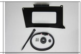
FMS Accessory radio receiver relocation kit mounting bracket should fit most agency receivers with a width of 7" between the mounting points. Secure with screws provided with the radio receiver chassis, with the antenna and power connections facing the rear of the saddlebag.
